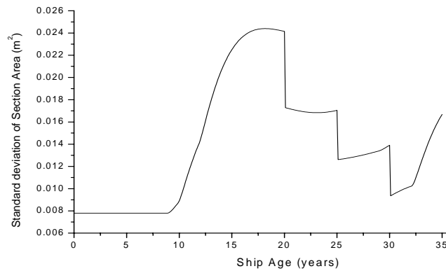
Fig.5 Standard deviation of the midship section modulus as a function of time
