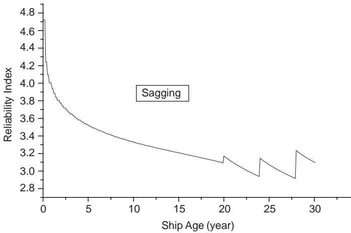
Fig. 15. The reliability index based on sagging ultimate bending moment.
